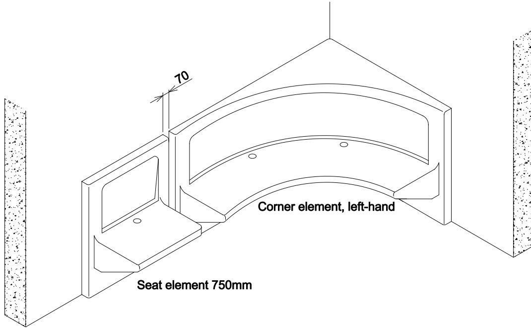
**Step 1 :** Mark the positions of the fixing holes on the wall.
