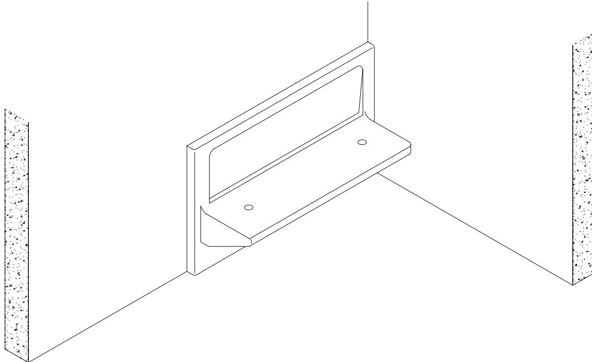
Mark and drill the Ø8mm fixing holes in de wall
