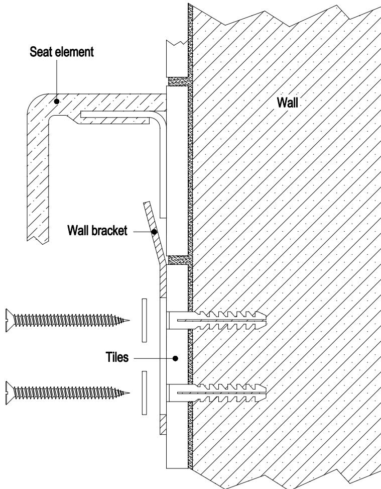
The plugs supplied in the kit are intended for use in concrete/solid stone walls.
