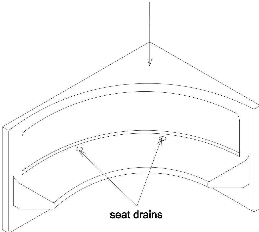
**Maximum load capacity** of the seat elements is 100 kg per single-person seat position.
